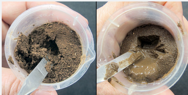
Figure 6: Structured soil (left) processed at 2 mm that has been moistened by capillary action and is not over-wetted; unstructured soil (right) that was processed to < 0.8 mm and wetted by capillary action and became too moist for respiration test.
